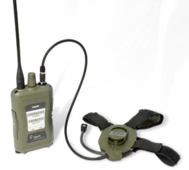
The FSR has a modular architecture and can be equipped with up to two RF transceivers. The current implementation includes a PRR/EZPRR compatible module, and either the Soldier Broadband Waveform (SBW) or Soldier Narrowband Waveform (SNW) modules. The architecture enables future incorporation of user-defined waveforms.
